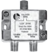
The LUV-2150 is a L-Band diplexer used to combine or separate UHF/VHF/CATV frequencies (10 to 806 MHz) and L-Band satellite signals (950 to 2150 MHz).
